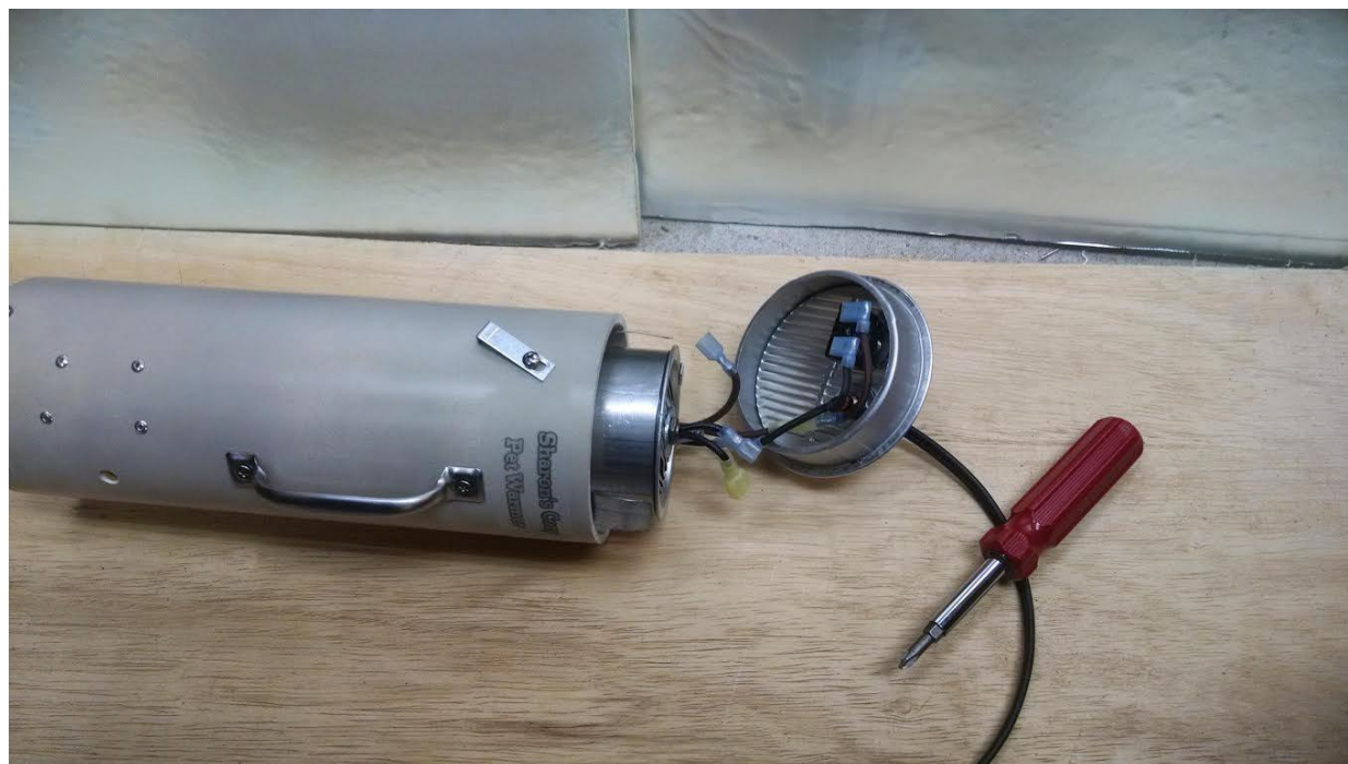
Figure 3 (Removing Inner Retaining Screw):
