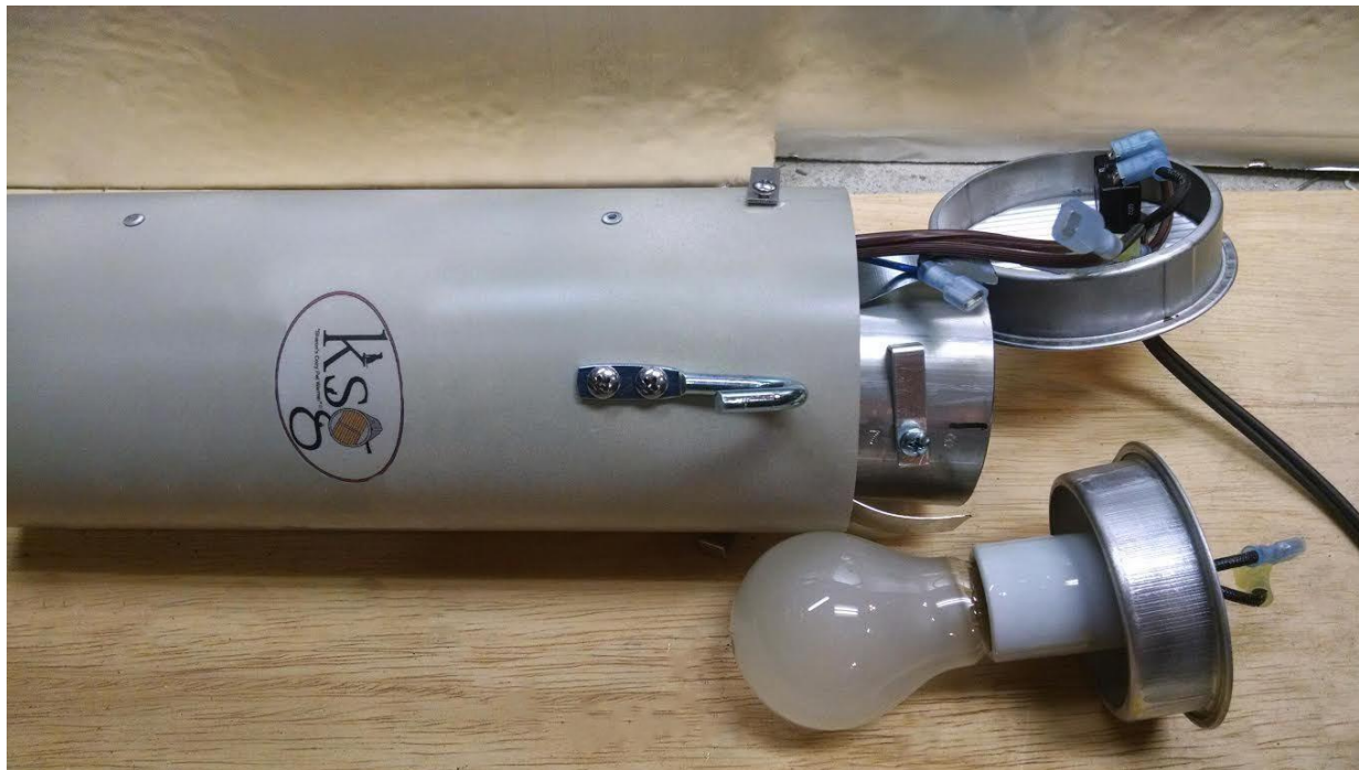
Figure 4 (Exposing and Replacing Heating Element):
